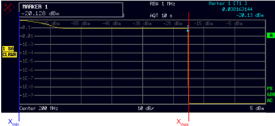
Fig. 4-19 APD of a pulsed signal (high PRF)
